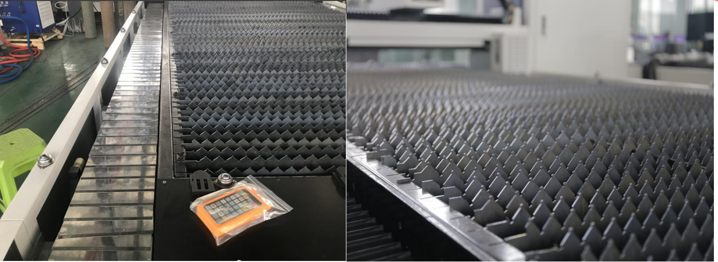
11. Sawtooth blade table ,suitable for cutting any material , also can easy change future
